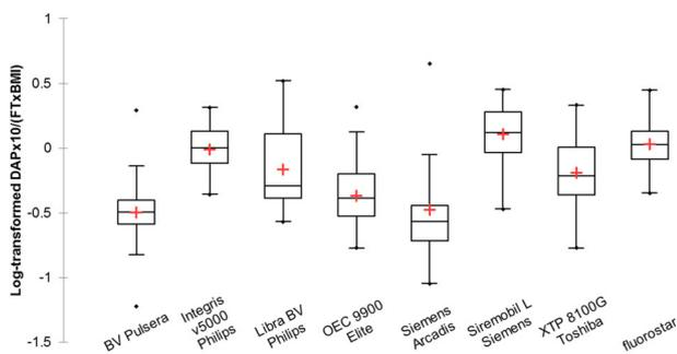
**FIGURE 3** Comparison of radiation dose among generators: distribution of log-transformed  $\frac{\text{DAP} \times 10}{\text{BMI} \times \text{FT}}$  per generator for single and dual chamber procedures [Color figure can be viewed at [wileyonlinelibrary.com](http://wileyonlinelibrary.com)]
